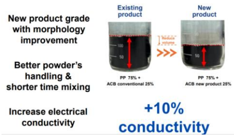
Figure 2. High-dispersibility ACB production by cracking furnace improvement
