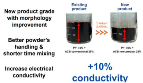
Figure 2. High-dispersibility ACB production by cracking furnace improvement
